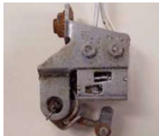
Treated with SuperCORR A after 1,400 hours
